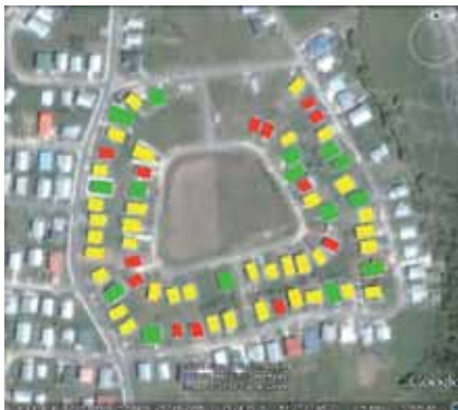
Sample output of a vulnerability assessment based on satellite observations. A "vulnerability" tag, represented by a colour in a "vulnerability palette" ranging from green (least vulnerable) to red (extremely vulnerable), is attached to the examined buildings shown on a GoogleEarth image
